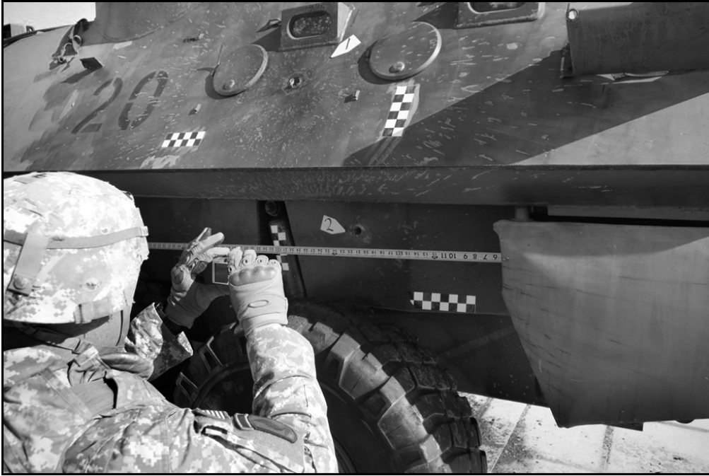
Figure G-35. Exterior photograph of damaged area using rulers
